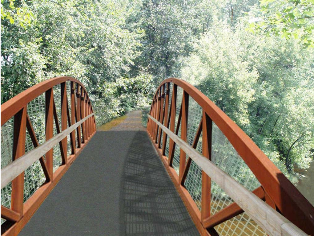
Figure 47: Alternative 3 - Prefabricated Bridge (Truss Type)
